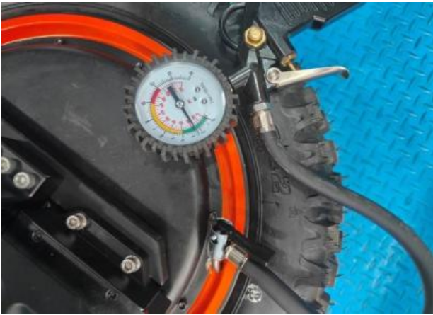
22 Tire pressure test
