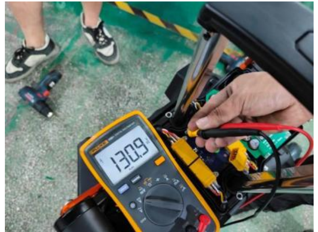
Actual Checked Battery Voltage against Voltage by App
