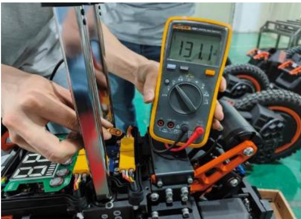
12 Full battery voltage check
