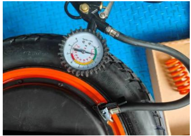
21 Tire pressure test
