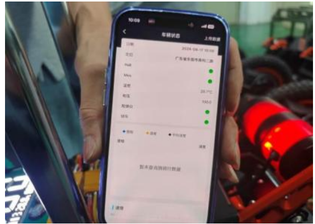
11 Full battery voltage check
