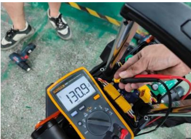
18 Full battery voltage check
