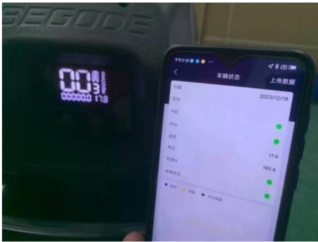
Battery voltage check By App:
