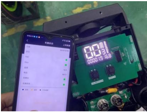
Battery voltage check By App:
