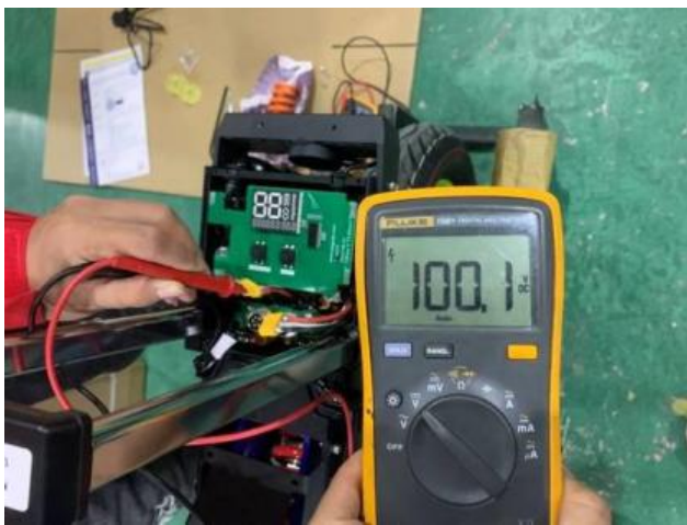
Battery voltage check
